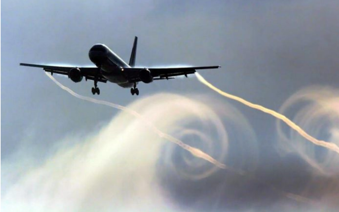
Figure 3.12: Jet-induced flow separation leading to crosswise (spanwise) vortex rolls in its wake and streamwise vortices at their core.
