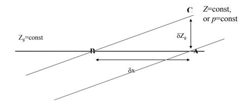
$$\left(\partial_{x} p\right)_{Z_{g}} = \frac{p_{A} - p_{B}}{\delta x} = \frac{p_{A} - p_{C}}{\delta x} = \frac{g\rho(Z_{g_{A}} - Z_{g_{C}})}{\delta x} = \frac{g\rho(Z_{g_{B}} - Z_{g_{C}})}{\delta x} = \rho\left(\frac{\partial \Phi}{\partial x}\right)_{Z_{g}},$$
