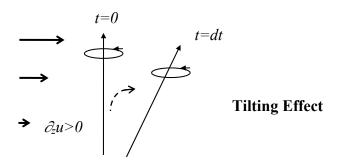
The tilting effect changes the direction of the vorticity. Consider a vortex tube, originally assumed in the z direction. The shear flow will tilts it down the direction of the shear,
