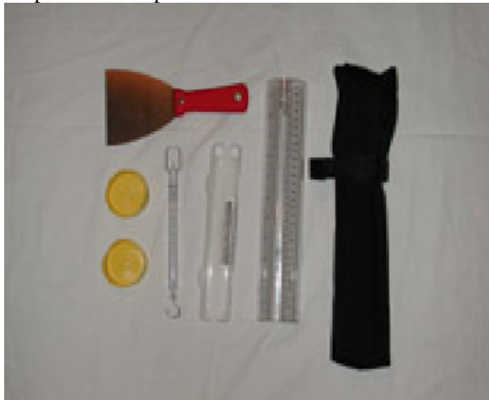
Figure 2. Snow Density sampling kit provided by SPL. Includes scale, sampling tube, and shovel.
