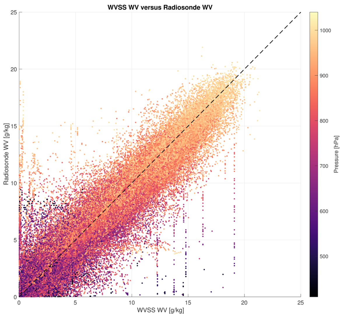
Figure 4.1: WVSS-II water vapor mixing ratio value with matching radiosonde water vapor mixing ratio value plotted with color scale indicating pressure level of the match.
